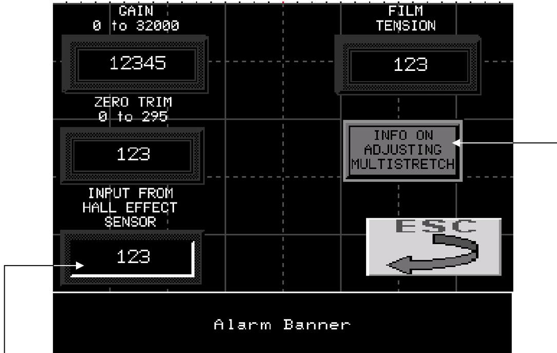
Feedback value from the hall effect device is useful for troubleshooting. It shows a real-time signal value from the hall effect so that the ZERO setting can be calibrated.
