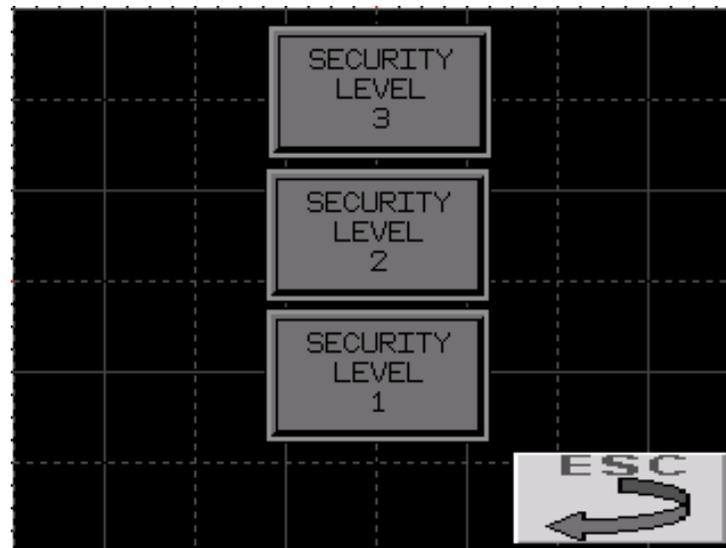
**Security Level #1** removes most lockouts. All major settings (wrap counts, carriage speed, tension etc are open). Timers are still adjustable.
